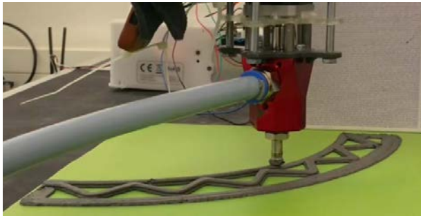
Figure 8. Clay print using the implemented robot control system. The shown clay extruder nozzle is mounted on a UR10e robot.
